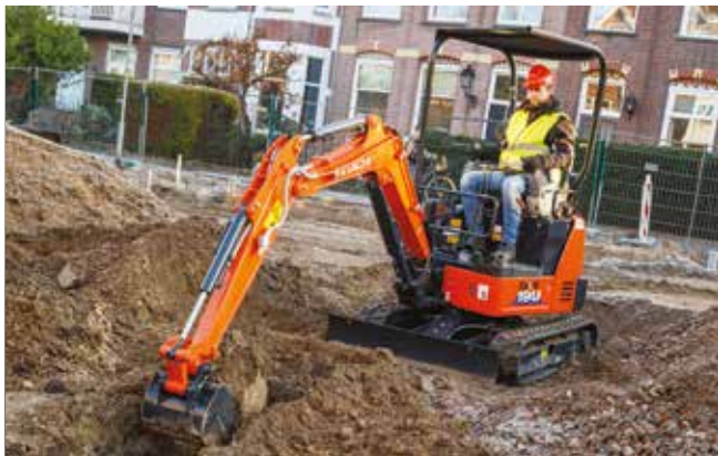
Expandable crawler tracks enhance versatility and stability.
