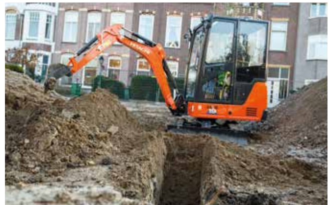
The boom cylinder on top of the boom minimises downtime due to reduced contact with the cylinder.
