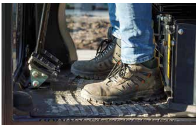
Folding travel pedals can be used instead of a hand lever.
