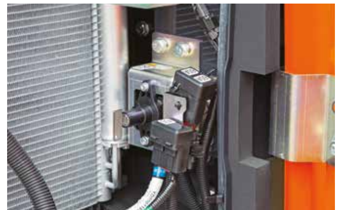
The battery disconnect switch allows maintenance to be carried out safely.
