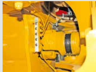
The centralised lube bank places difficult-to-reach grease points within reach.
